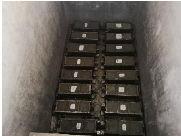
Figure 1: Samples in the deep freezer exposed to frost
