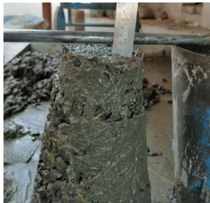
Figure 2: Measuring slump of HNFRC.
