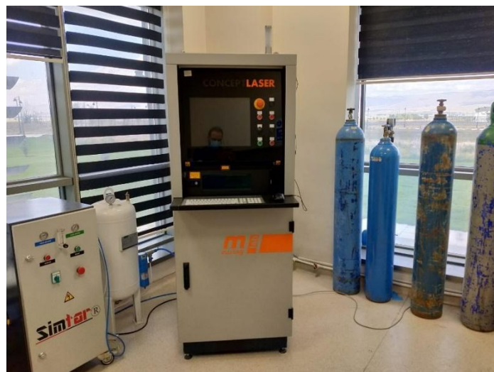
Fig. 1: Concept Laser M Lab R SLM device
