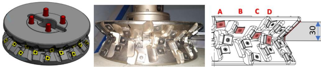
Şekil 2 : Beveling tool a-3D model, b-Tool photo c-position of sheet metal plate and cutters
