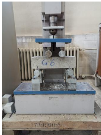
Figure 1. Four-point flexural test
